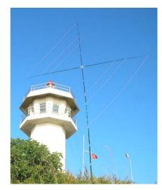
1el Quad 20/15/10 on 12m fiberglass pole
