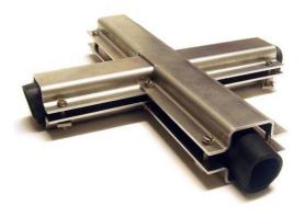
The metal center cross is constructed of two 2 aluminium angles "type A" (200mm long, no cut-outs) and 2 aluminium angles "type B" (240mm long, with center cut-out). Stick them together as shown in the photo and attach the screws. As the square nuts are self-blocking against the aluminium angle, it is easily possible to assemble the metal cross from only one side, needing just a single screwdriver.
