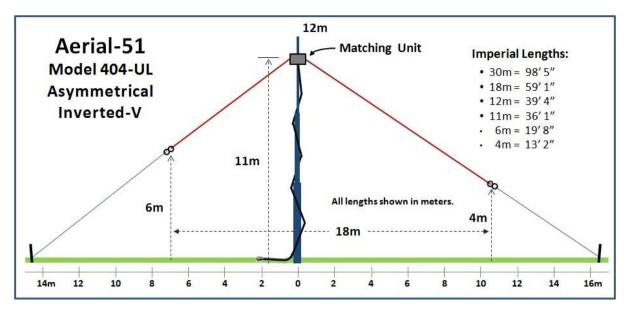
The Model 404-UL is a half wavelength long wire antenna on 40m. Though it uses a different feedpoint position, it works similar to a classical OCFD or dual-wire fed Windom. Whereas the original Windom design only covers even harmonic bands, the 404-UL was designed to also cover odd harmonic bands.
