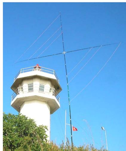
1el Quad 20/15/10 on 12m fiberglass pole
